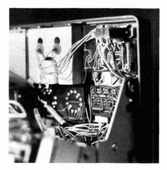
fig. 4A. Dim switch circuit board.
